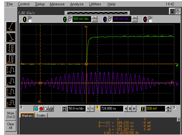
Figure-3 : delay 1pps TX – 70 IF MHz output
